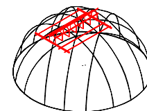
Figure 8 – Nest and Roost Pole System Suspended from Ceiling
